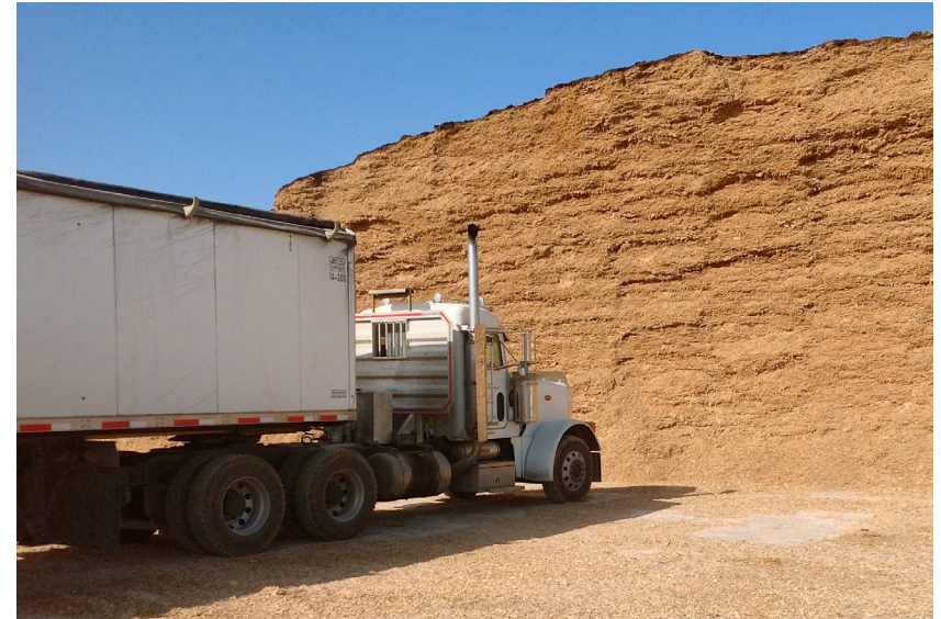
Figure 8. Silage truck parked too close to the feedout face
