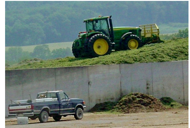
Figure 1. Pack tractor operator in dangerous position above the bunker silo wall
