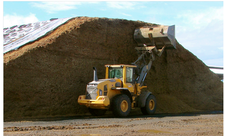
Figure 9. Payloader operator removing silage from an over-filled bunker silo
